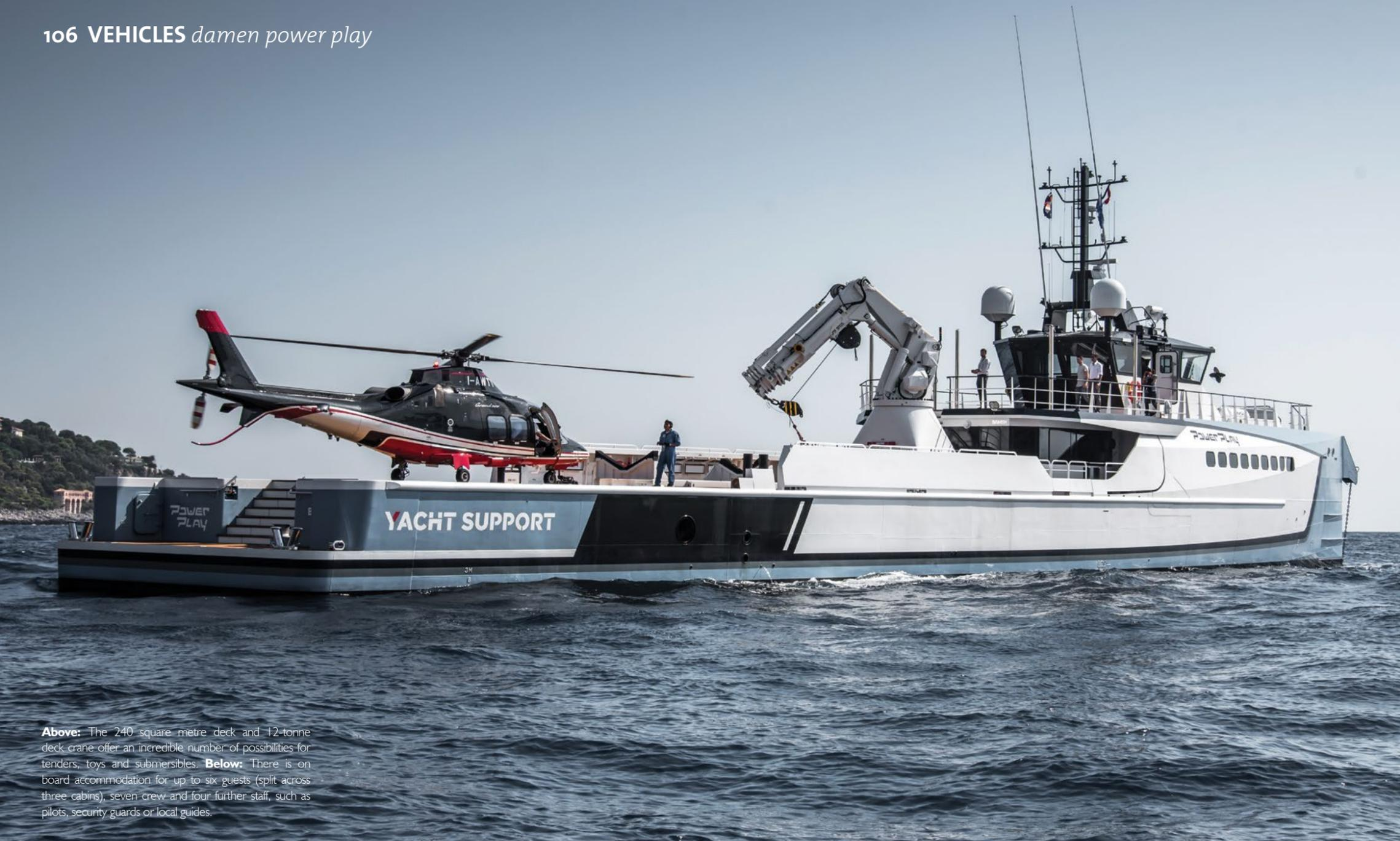
**Above:** The 240 square metre deck and 12-tonne deck crane offer an incredible number of possibilities for tenders, toys and submersibles. **Below:** There is on board accommodation for up to six guests (split across three cabins), seven crew and four further staff, such as pilots, security guards or local guides.
